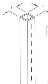
\*1"x 2" slotted tube standard also available with slotting on one or both 1" sides. Part number 880.
