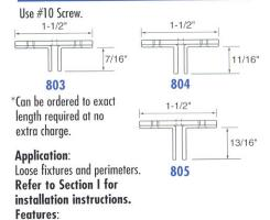
1/6" thick steel. On center dimension from counter-sunk screw hole to counter-sunk screw hole is 6" staggered side to side
